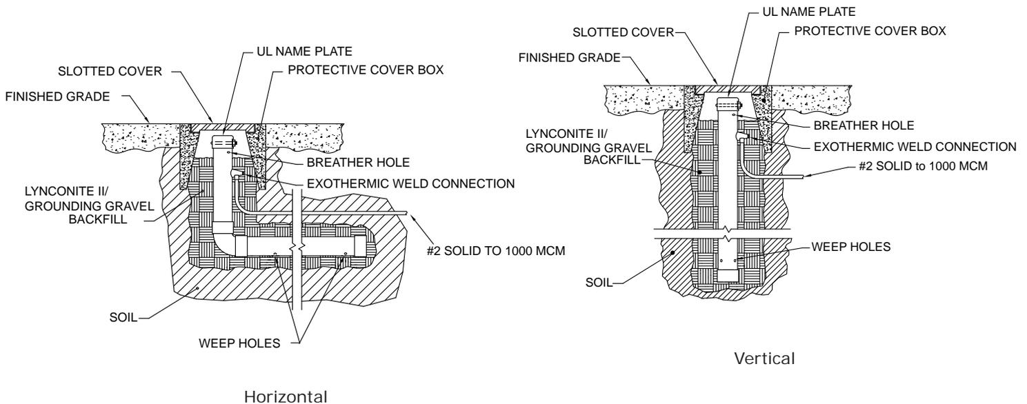
**Features:** Kit includes the chemical electrode (filled with electrolytic salts), bentonite, 50 lb. of Contact-GM backfill, and an inspection well.
